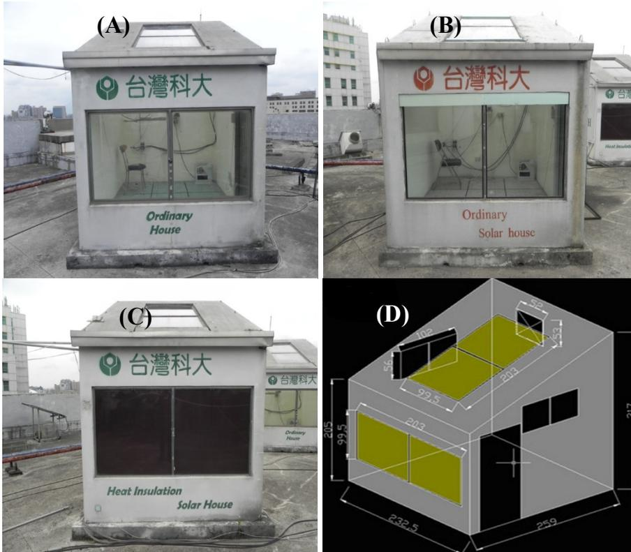
**Fig. 3: Outside appearance of experimental houses: (A) Ordinary House, (B) Ordinary Solar House (Low-E house) and (C) HISG House were installed by normal glass, Low-E glass, and HISG; and (D) 3D perspective, respectively**
