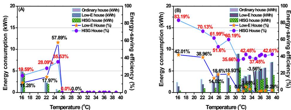
Fig. 5: Energy-saving efficiency for (A) Heating and (B) Cooling of the experimental houses with different temperature
