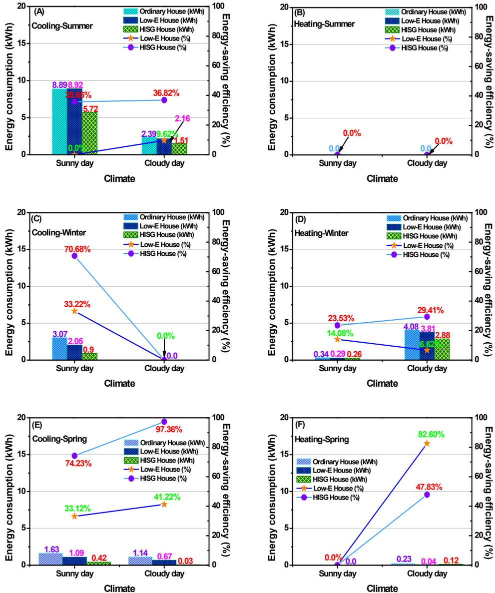
Fig. 4: Electric energy consumption of Ordinary house, Low-E house and HISG house during different seasons of (A, B) Summer; (C, D) Winter; and (E, F) Spring for cooling and heating in sunny and cloudy days, respectively
