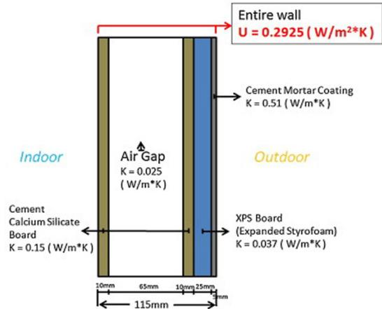
**Fig. 2: Thickness and thermal conductivity of all elements of the external envelope of the experimental houses**
