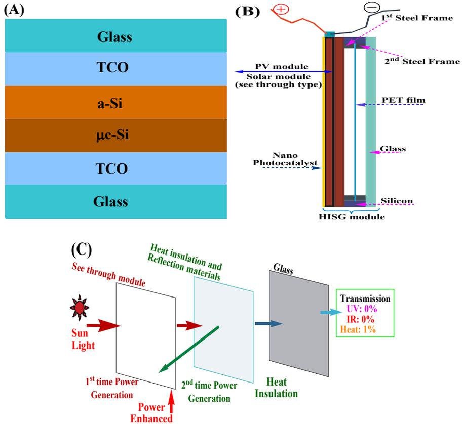
Fig. 1: Structures of (A) original PV module and (B) HISG module (thickness ~28 mm), and (C) Scheme about function theory of HISG
